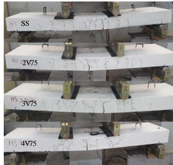
Figure 12. Effect of longitudinal voids number on crack pattern of hollow-core high strength slabs
