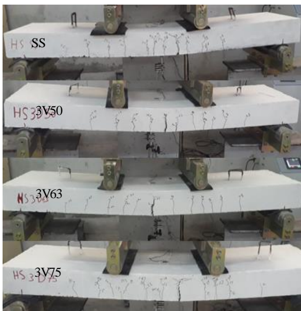
Figure 11. Effect of longitudinal voids diameter on crack pattern of hollow-core high strength slabs
