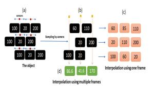
**Figure 3.** A simple example to illustrate single-frame interpolation vs. multi-frame interpolation. a) The object which it was imaged, b) Sampling by camera sensors, c) interpolating using one frame. The middle pixel is the average of the neighboring pixel, d) multi-frame interpolation. Green pixels are the weighted average of the pixels that hit the yellow line.
