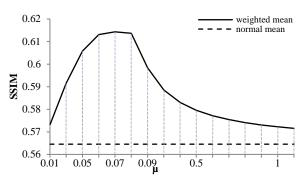
Figure 14. The effect of  $\boldsymbol{\mu}$  on distance Equation (2) on the SSIM
