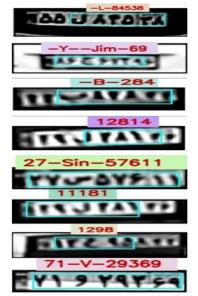
Figure 15. The license plate recognition using OCR
