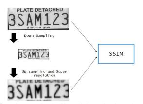
**Figure 9.** Measuring the SSIM criterion using the produced super-resolution and the reference image
