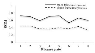
Figure 10. SSIM criterion for super-resolution using the proposed multi-frame and ordinary single-frame interpolation
