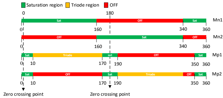
Figure 3. Transistors operation region in a period for the oscillator of Figure 1
