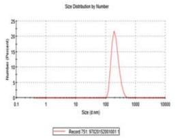
Figure 3. DLS Analysis of Fe<sub>3</sub>O<sub>4</sub>/CMC Nanoparticles
