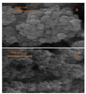
**Figure 2.** (a) SEM Images of Fe<sub>3</sub>O<sub>4</sub>/CMC in 15 kV-200 nm, (b) SEM Images of Immobilized Laccase 15 kV-500 nm
