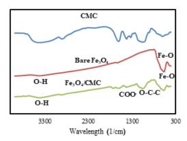
Figure 1. FTIR Spectra of CMC, Fe<sub>3</sub>O<sub>4</sub>, Fe<sub>3</sub>O<sub>4</sub>/CMC
