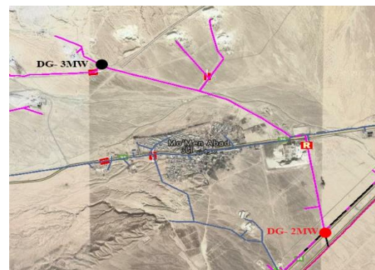
Figure 3. The optimal location of the allocated DER in feeder 5 based on two algorithms
