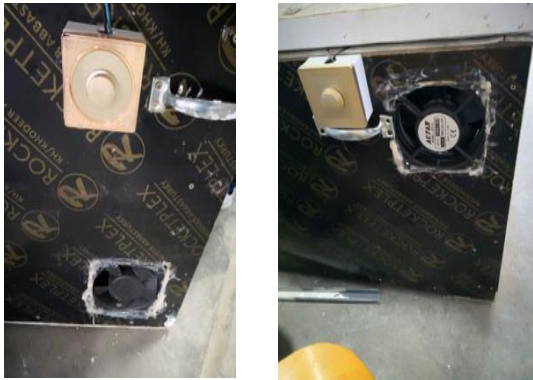
Figure 2. Intake and outtake fans
