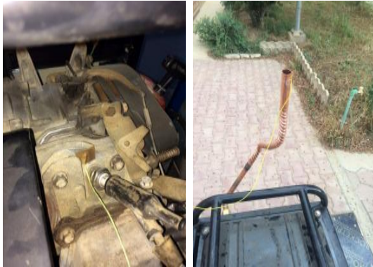
Figure 4. Fixing thermocouples at engine cylinder head and at exhaust
