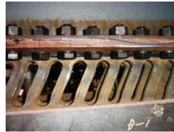
Figure 10. Damper deformation of D1 specimen [27]
