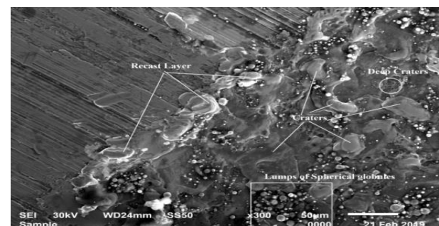
Figure 11. SEM image at X300 magnification for Pongamia pinnata oil workpiece
