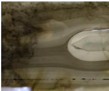
Figure 4. A view of the flow pattern around the wedge model
