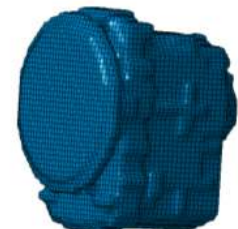
Figure 5. The boundary element model of the gearbox
