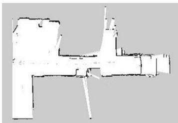
Figure 17. The final merged map obtained by using the proposed merging algorithm (first test)
