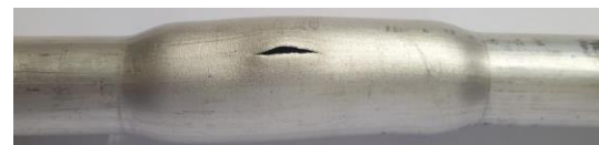
Figure 9. Incomplete stepped tube in the HHB process at room temperature ( \lambda=26 %)
