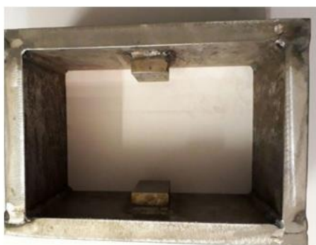
Figure 11. Iron core to prevent the dispersion and leakage of magnetic flux (polar spacers are welded to the core yoke)
