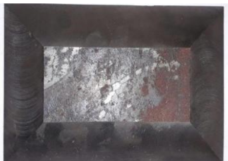
Figure 12. A slanted piece which is used to simplify the installation of PM parts and to improve the magnetic field
