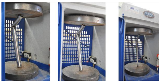
Figure 8. Buckling in quarter height
