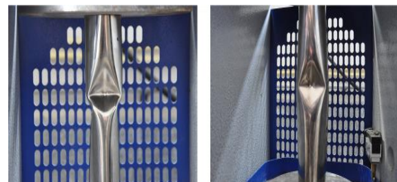
Figure 6. Diamond shape failure
