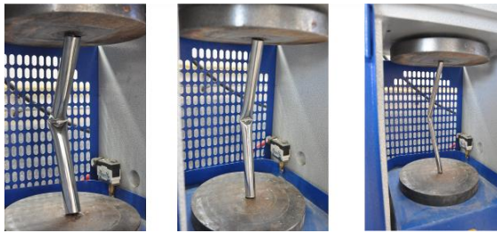
Figure 7. Buckling in mid height
