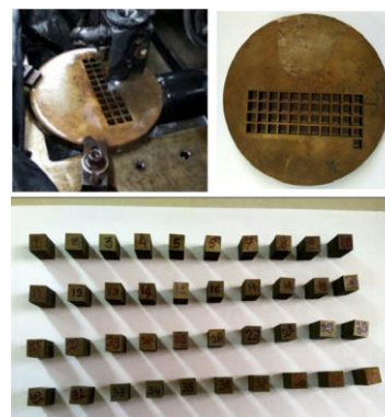
Figure 2. Complete job after WEDM
