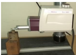
Figure 1. Set up for Surface roughness measurement
