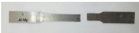
Figure 2. Al-Mg alloy standard tensile specimen after testing
