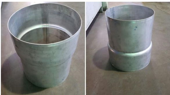
Figure 4. Cold bulge formed Aluminium blank after bulge forming process using polyurethane medium
