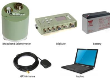
Figure 2. Tools and equipment of microtremor survey
