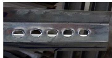
Figure 3. Deformation of 10 mm initial hole diameter
