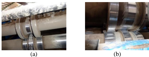
Figure 2. a) 1 st stage b) 5 th stage of the roll forming machine
