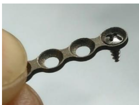
Figure 1. Ti-6Al-4V implant miniplate manufactured by EDM [15]
