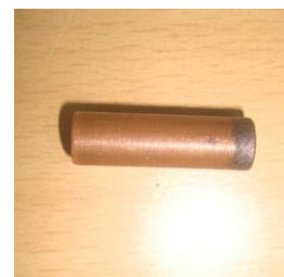
Figure 3. Tool used for machining of Hastelloy C-276
