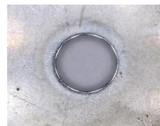
Figure 4. Machined hole using EDM in Hastelloy C-276
