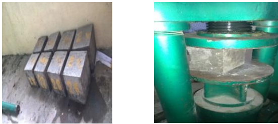
Figure 2. Testing on cubes for finding compressive strength
