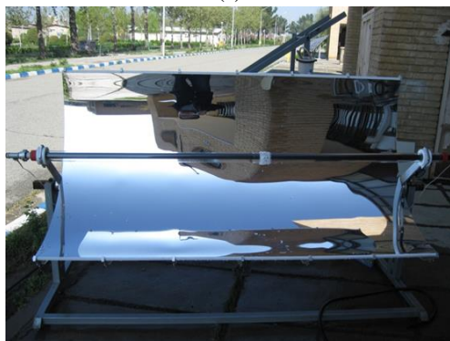
Figure 1. a) Schematic of closed loop test system for solar collector. b) parabolic solar collector trough
