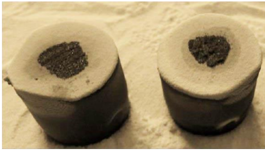
Figure 2. Corrosive salt on the coating surface
