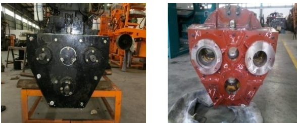
Figure 8. The transfer case before and after improvement
