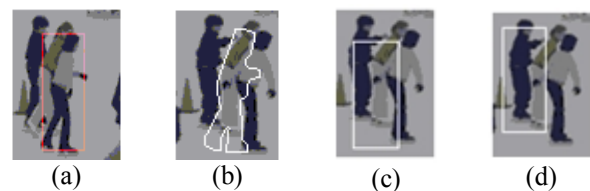
Figure 5. Original and asymmetric kernel mean shift tracking results when background information influenced the center of candidate model: (a) previous object region, (b) candidate model, (c) original mean shift method and (d) asymmetric kernel method.
