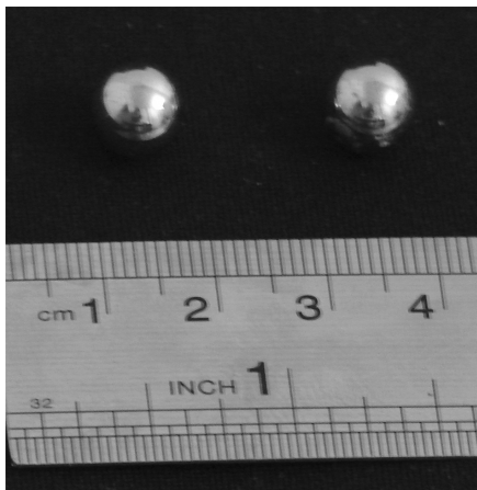
Figure 5. Stainless steel spherical ball projectile used for high velocity impact tests
