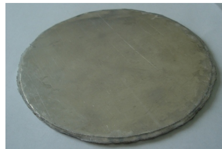
Figure 2. Image of the fiber-metal laminate specimen preparation.
