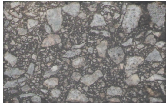
Figure 11. Vertically sliced Marshall hammer compacted specimen
