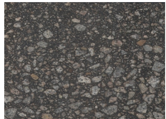
Figure 13. Vertically sliced Presbox compacted specimen
