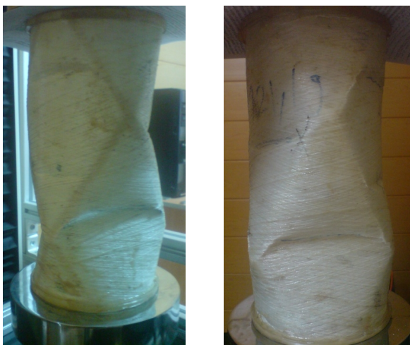
Figure 7c. Local buckling and failure mode of a complete shell
