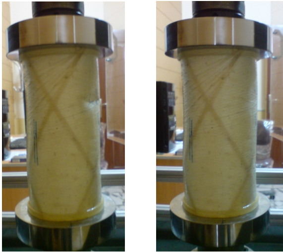
Figure 7a. Global buckling of defective sample
