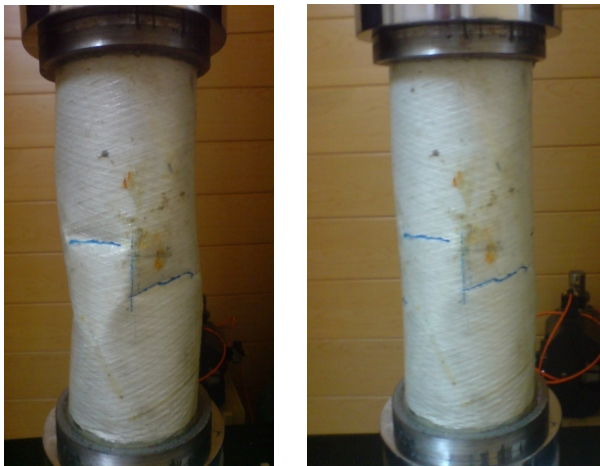
Figure 7b. Local buckling of defective sample
