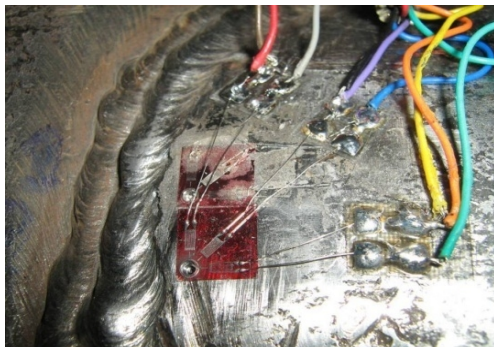
Figure 4. Residual stress measurement set-up
