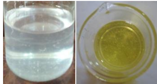
Figure 3. EG and transformer oil mixed with SiO 2 nanoparticles before sonication
