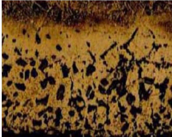
Figure 3. Optical micrograph of Fe-Ni particles in Fe-30 Ni-Cr-Al alloy after 25 hrs (X 1000).
