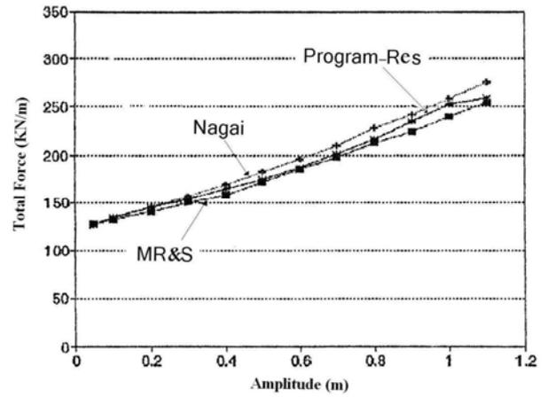
Figure 10. The variation of force with respect to amplitude.
