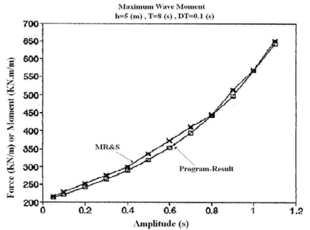
Figure 11. The variation of moment with respect to amplitude.
