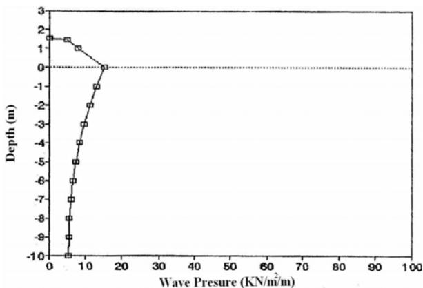
Figure 19. The net pressure of the wave for  $h = 10$ .
