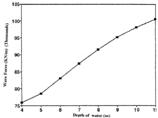
**Figure 16.** Variation of wave force due to the water depth.
