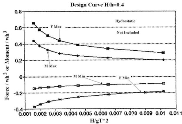
Figure 21. Design curves for  $H_i / h_i = 0.4$ .
