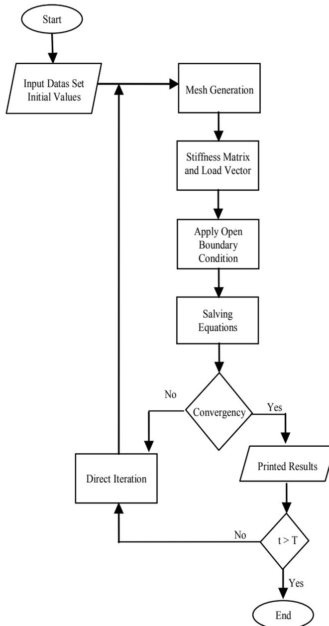
**Figure 22.** The flow chart of the finite element program.
