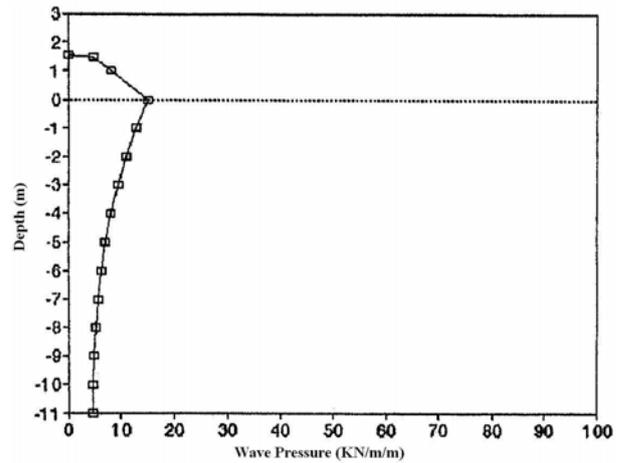
Figure 20. The net pressure of the wave for  $h = 11$ .
