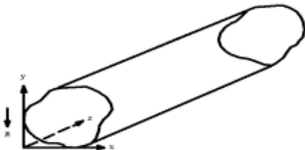
Figure 1. Arbitrary cross-sectional duct in Cartesian coordinates.
