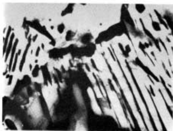
Figure 12. Transmission electron micrograph showing austenite-pearlite interface partially transformed at 690°C for 330 sec.
