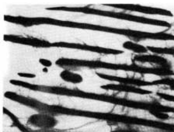
Figure 11. Transmission electron micrograph showing the trace of electron probe on cementite and ferrite lamellae, transformed at 660°C.
