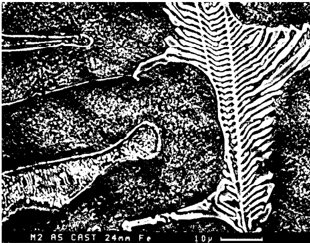
Figure 3. Cast structure of M2 HSS
