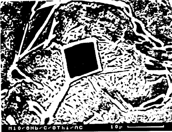
Figure 6. Cast structure of M10+NbC
