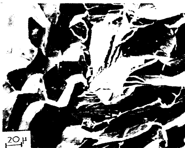
Figure 4. «River patterns» transgranular cleavage: 6.6 \times 10^{-3} \mu\text{m s}^{-1}
