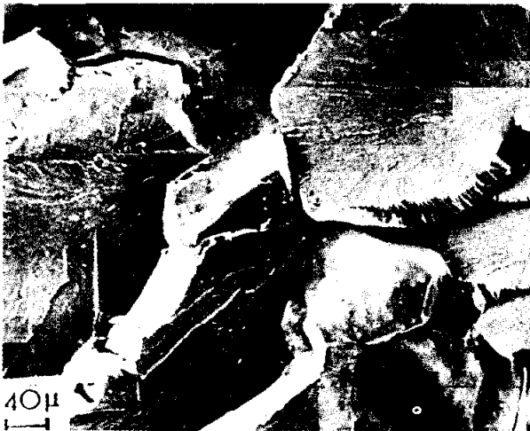
Figure 5. «Fan shaped» cleavage facets: 6.6 \times 10^{-3} \mu\text{m s}^{-1}
