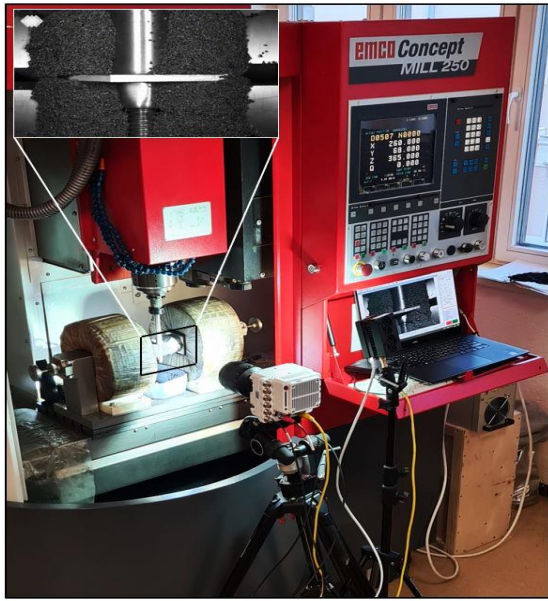
Figure 1. Experimental complex for abrasive finishing in a magnetic field
