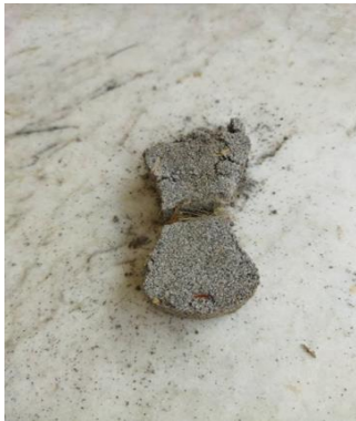
Figure 16. A fractured 8-shaped sample tested in this investigation
