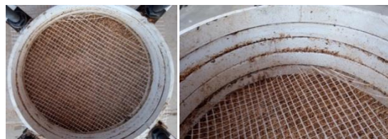
Figure 7. A ruptured sample of the blanket's geogrid reinforcement at the end of the test
