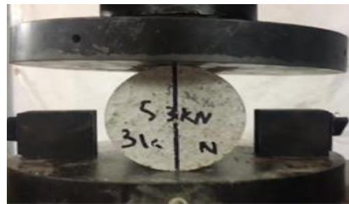
Figure 4. Failure sample of geopolymer concrete
