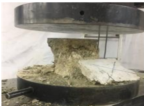
Figure 3. Failure sample of geopolymer concrete
