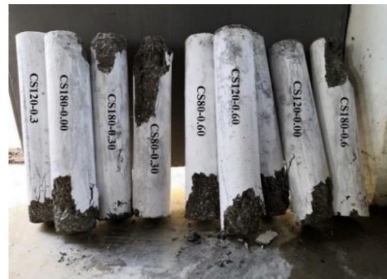
Figure 10. Failure patterns of short columns
