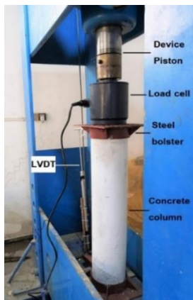
Figure 5. Test setup and instrumentation
