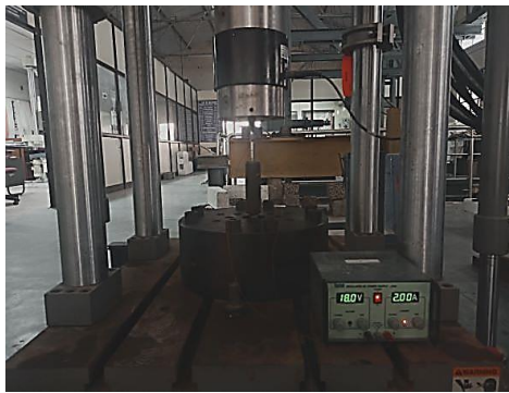
Figure 8. MR damper on the MTS loading frame
