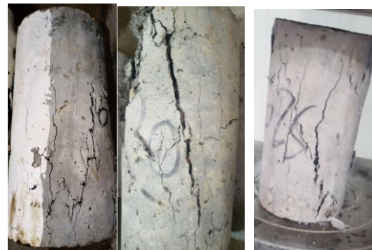
Figure 6. Failure mode of cylinders
