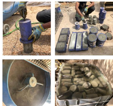
Figure 1. Casting and curing process
