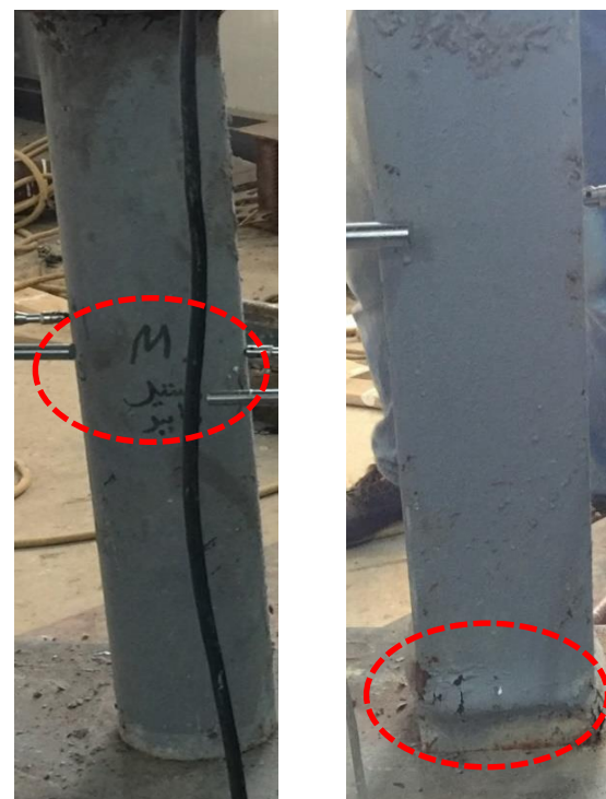
a) Circular column- local buckling at the mid-height b) square column- Local buckling at the column end
