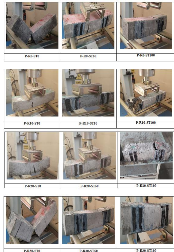
Figure 10. Failure observation of strengthening rubberized concrete prisms
