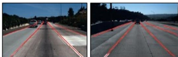
Figure 9. Sample output of lane detection using ResNet50
