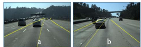
Figure 7. (a) Incorrect lane detection, (b) failure to accurately identify lane
