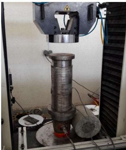
Figure 2. Applying preloading process on the fresh concrete
