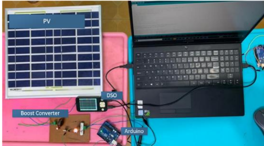
Figure 10a. Working model of PV MPPT system
