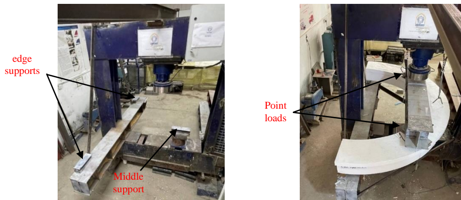
Figure 4. Test setup layout (a) Side view schematic drawing (b) Top view schematic drawing (c) photos
